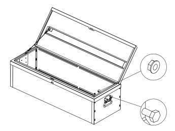
To assemble the lock, place the lock body in the opening on the front of the utility box. Thread the M18 hex nut onto the lock body, and tighten until the lock is secured against the front of the utility box. Slip-joint pliers can help tighten the nut into place.
