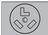
3-Wire Receptacle (NEMA Type 10-30R)
