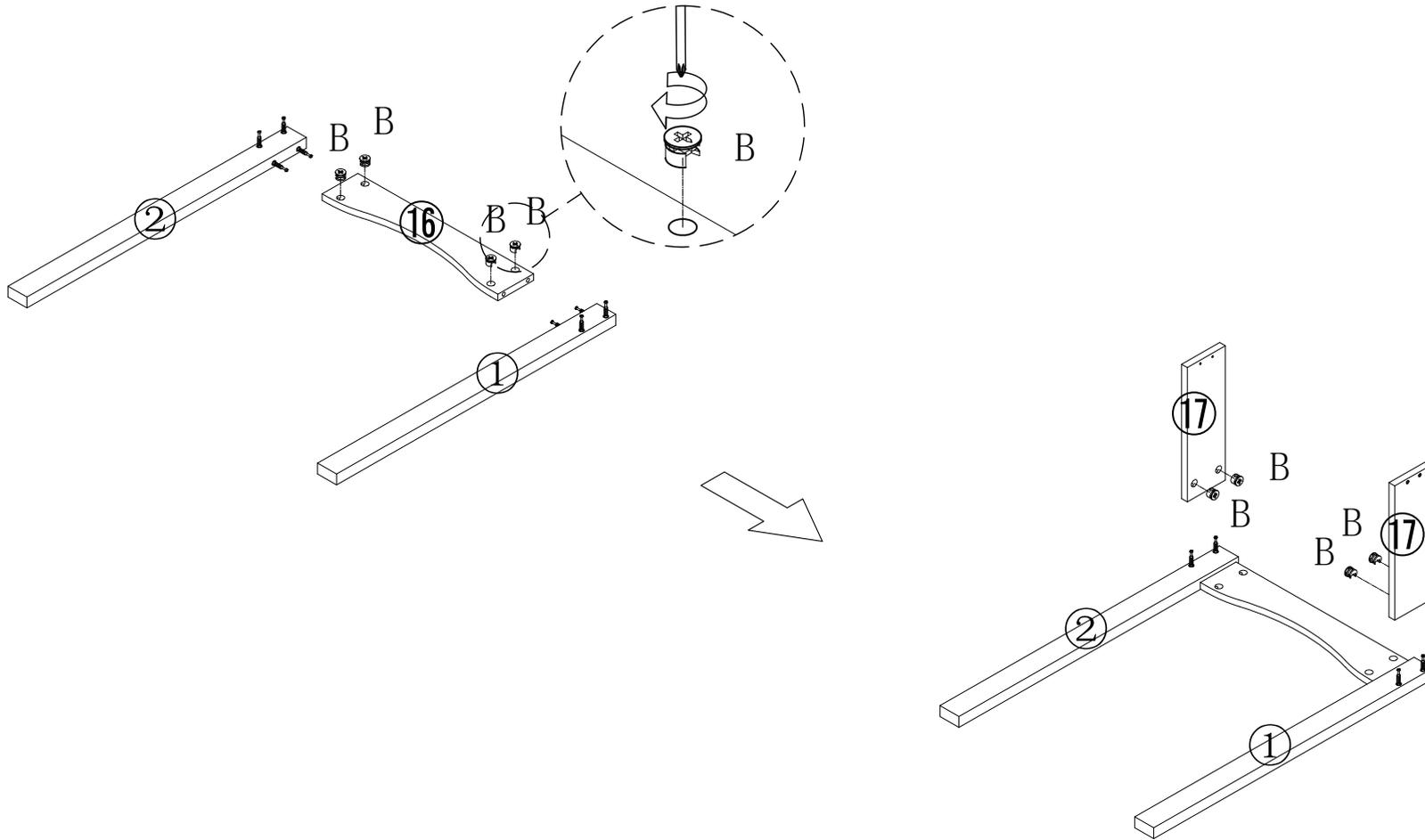
Make sure the arrow on the screw align to the hole on the side.
