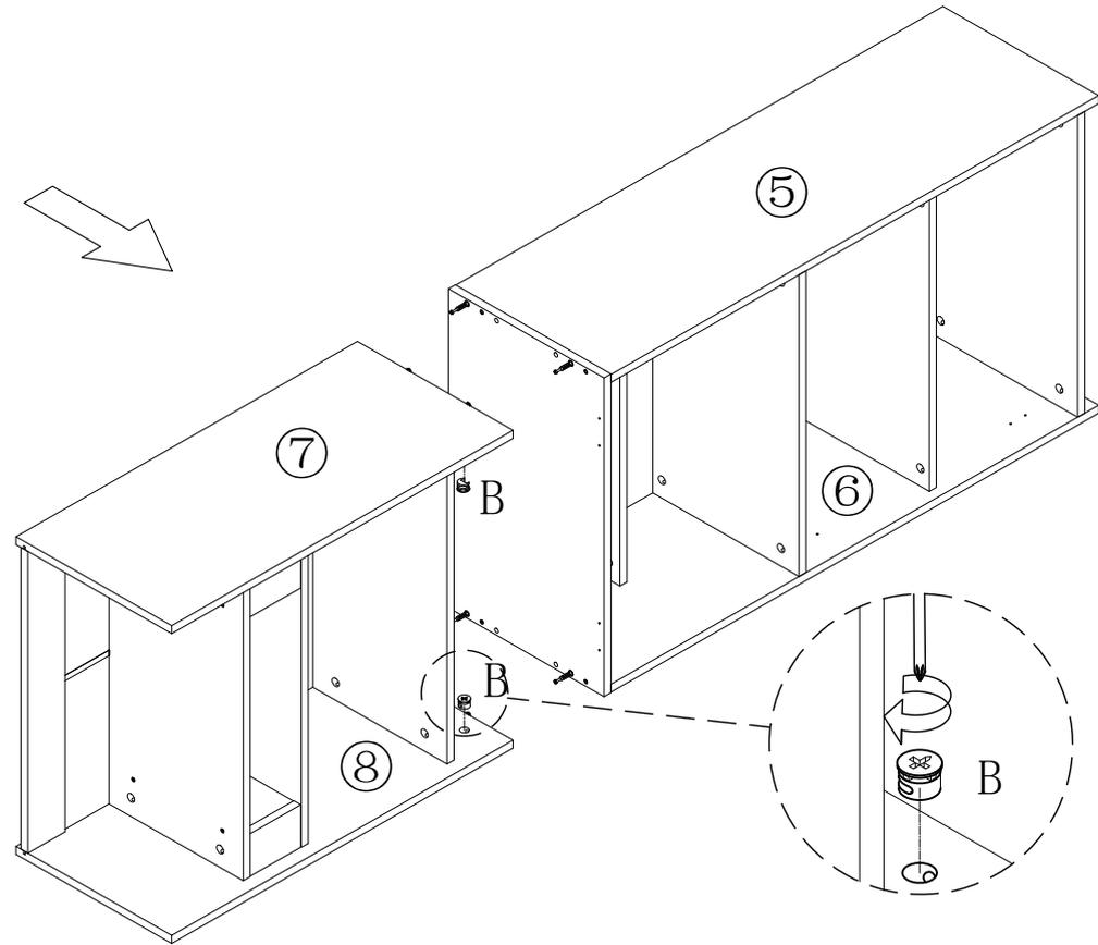
Make sure the arrow on the screw align to the hole on the side.
