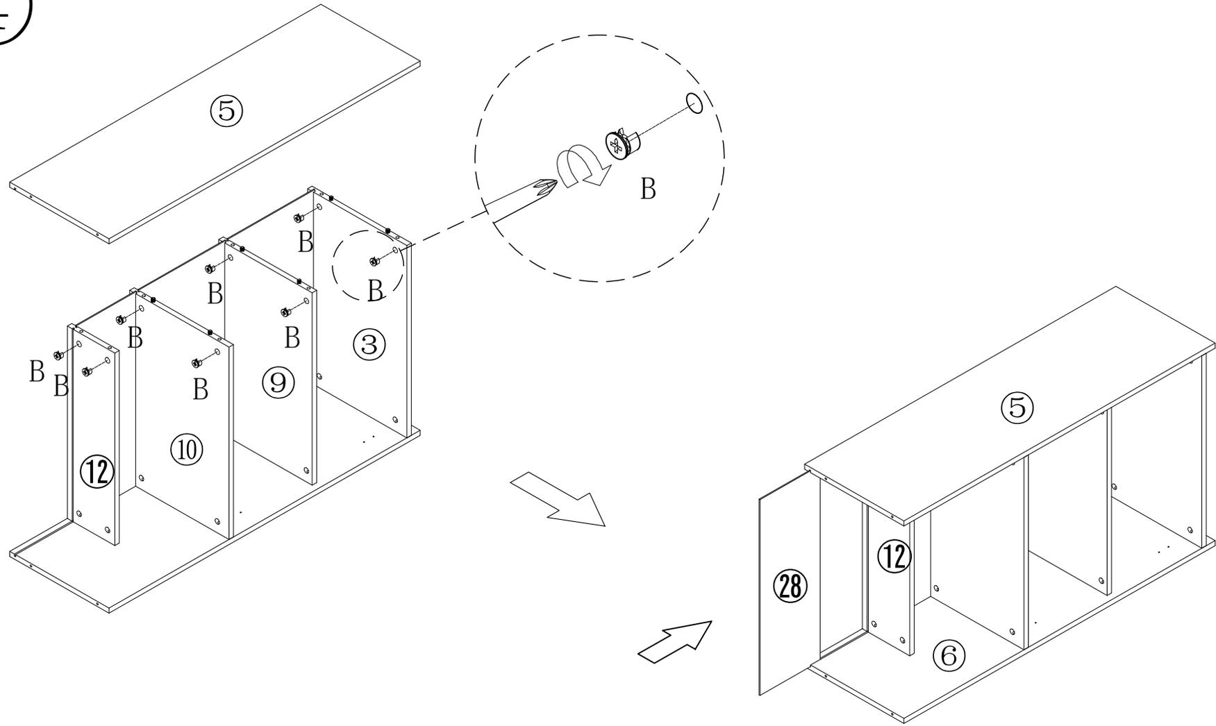
Make sure the arrow on the screw align to the hole on the side.
