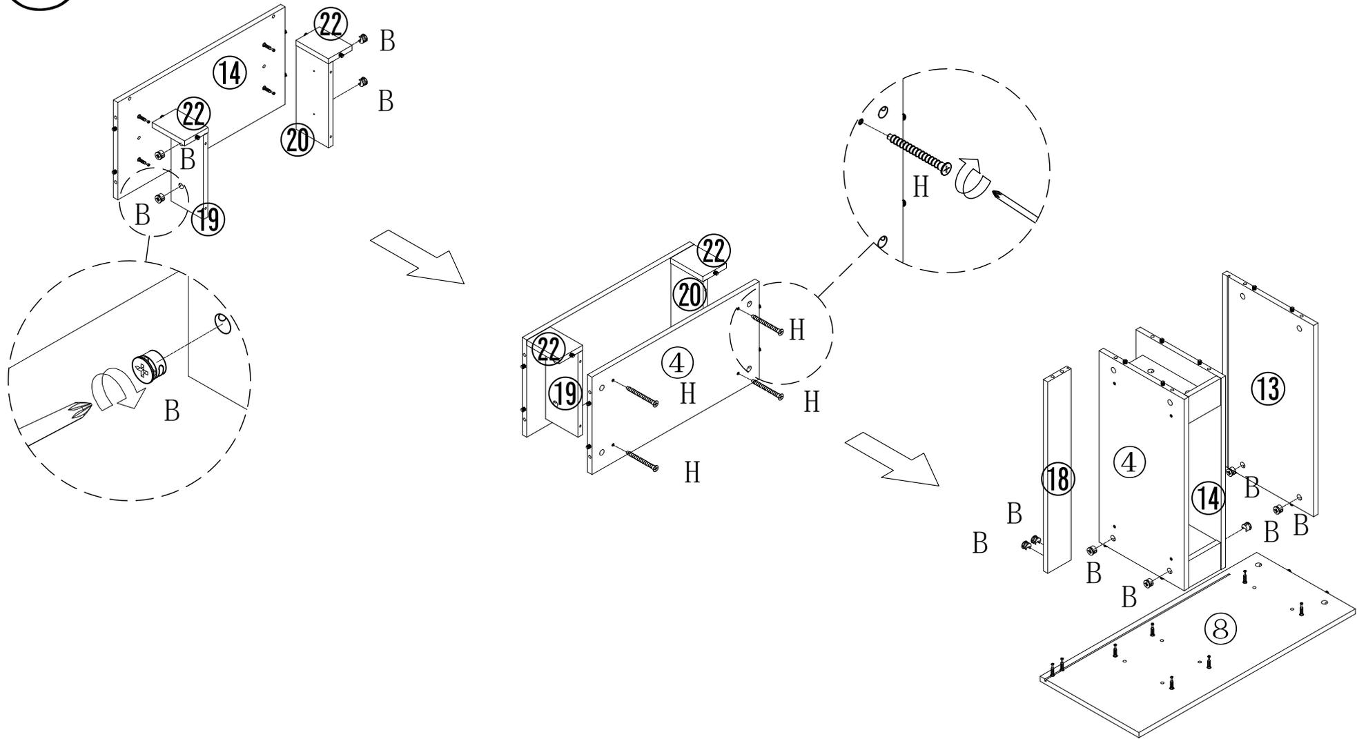
Make sure the arrow on the screw align to the hole on the side.
