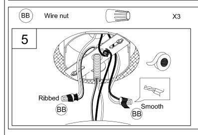
5. Strip 3/8" of insulation from the electrical wire ends. Using wire nuts (BB), connect RIBBED fixture wire to the WHITE supply wire from the outlet box; connect the SMOOTH fixture wire to the BLACK supply wire. Connect the fixture ground wire and supply ground wire using a wire nut or by fastening to the ground screw on the mounting strap. Push all wire connections into the outlet box.
