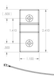
Tplug design allows for quick installation without using set screws to mount shower bar holder to wall bracket. No screws required to assemble wall mounting bracket to the shower bar holder. Easy tplug design allows you to just insert and rotate to connect
