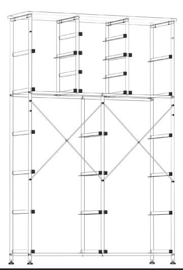
Be sure all curved ends (The place painted in black as shown in the figure) should be on one side to stop the drawers.
