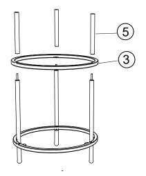
1. Place final frame 3 onto unit and screw ball ends 2 into short poles 5.
