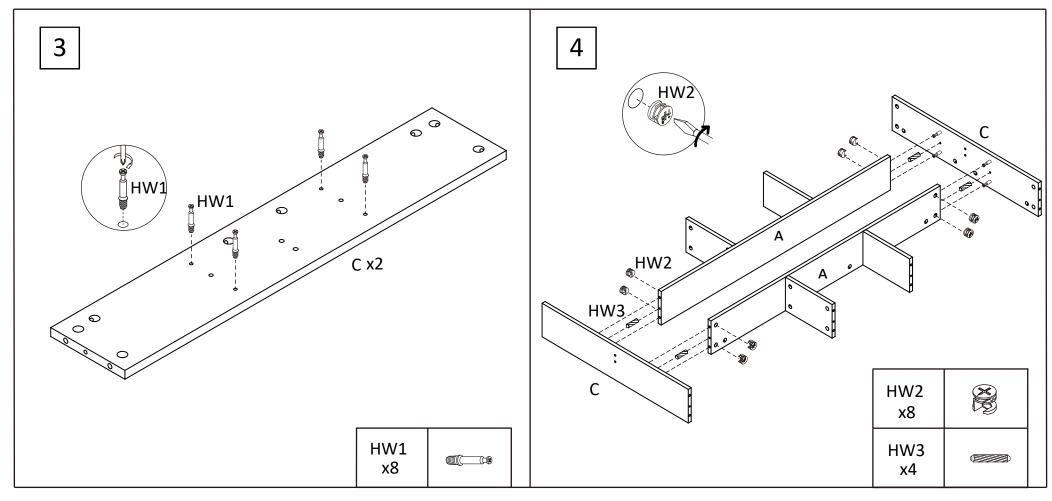
STEP3: Insert 8x cam bolts (HW1) into panel [C]. Tighten with a screwdriver. STEP4: Attach panels [C] to panels [A] with 4X dowels (HW3) and secure with 8x cam lock (HW2). Tighten with a screwdriver.
