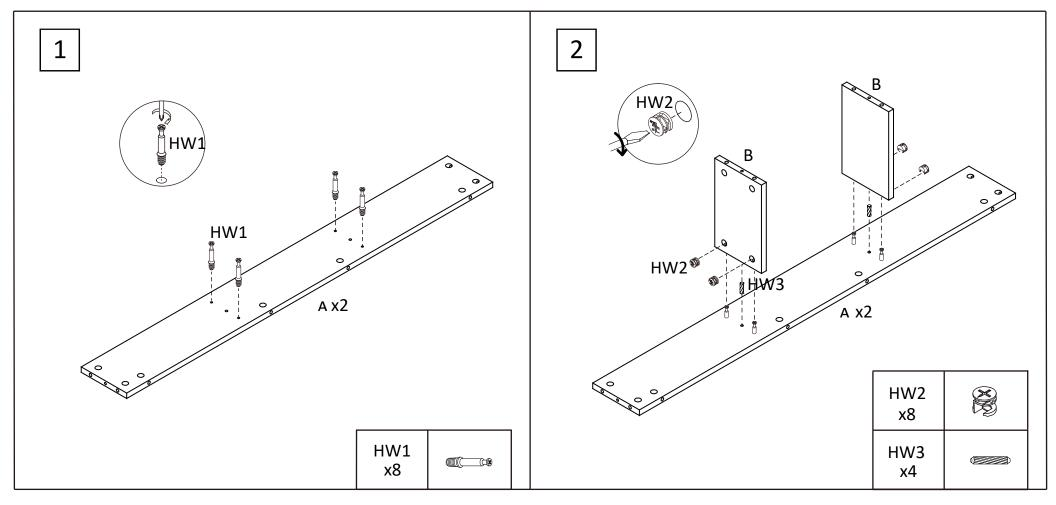
STEP1: Insert 8x cam bolts (HW1) into panel [A]. Tighten with a screwdriver.
