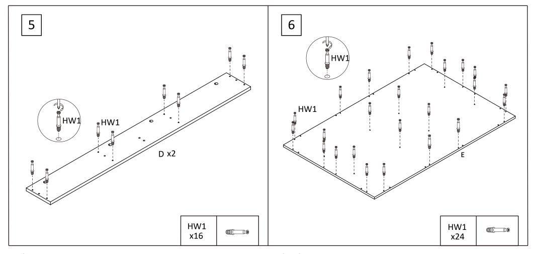
STEP5: Insert 16x cam bolts (HW1) into panel [D]. Tighten with a screwdriver. STEP6: Insert 24x cam bolts (HW1) into panel [E]. Tighten with a screwdriver.
