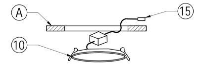
1. First, turn off the power at home. After turning off the power at home, put on insulating gloves to handle it. Connect the wires of the lamp and the wires at home through component #15 (insert several wires into the slot of component #15), and you can use it.
