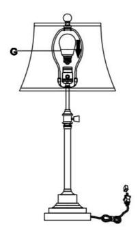
Step2 Insert the bulb(G) into the socket(C).
