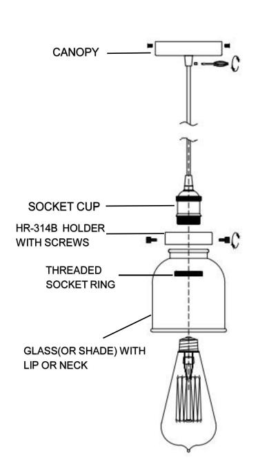
CHOOSE THE WIRE NEEDED FOR THECEILING HEIGHT, THEN FEED THE WIRESINTO THE CANOPY, THEN USE A SCREWDRIVER TO SCREW THE PLASTICSCREWS IN TO SECURE THE WIRES, AND THE PLASTIC STRAIN RELIEF IN THE CANOPYIS ALSO FIXED THROUGH THE WIRES.
