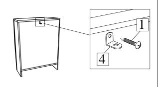
Locate the other bracket on the wall over a wall stud and two inches below the mounting bracket secured to the back of chest. Attached to the wall stud using the long screw provided, through the smaller hole
