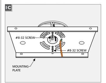
Secure the mounting plate to the electrical box with the two #8-32 screws provided.
