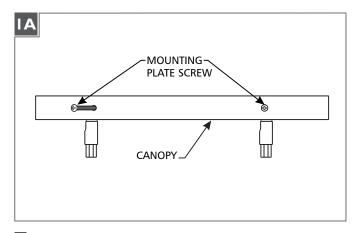
Separate the mounting plate assembly from the canopy by unscrewing the four mounting plate screws on the canopy.
