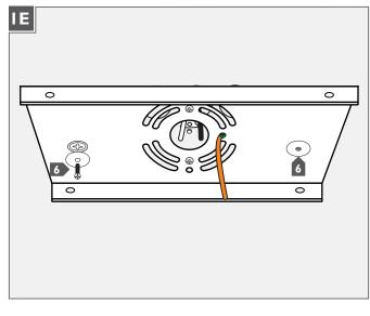
Secure the backplate to the anchors with screws and washers.
