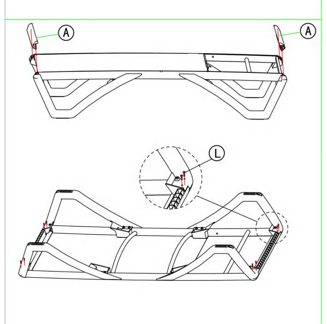
Turning it around,attach part A to the legs using Screws L.
