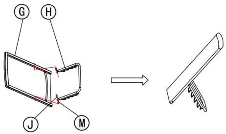
Please note: The Plastic cylinder Part M must be between Part G and Part H.
