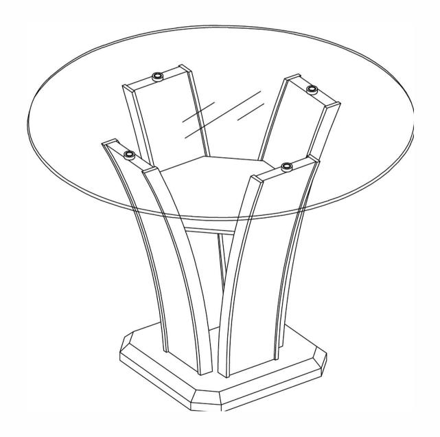
Do not tighten screws until completely assembled.
