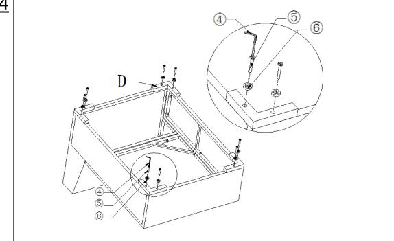
Attach the Feet(D) to the Chair using Bolt(5) and Washer(6) with Allen Key(4) as shown above.
