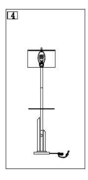
Step 1 Unpack all parts from cartons carefully. Check and make sure all parts are preser Insertlamp holder pipe(E) into tube(E Put the shade(J) on the Harp(I), then Insert tube(B), tube(D) into glass pane(C)
