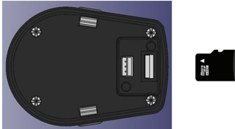
6. Once in place, lightly press the Micro-SD card into the camera module until you hear a slight click. Then release your finger. The Micro-SD card should bounce back slightly, but still be firmly in place in the camera module.
