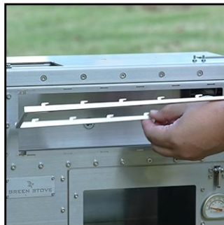
Take out the glass frame of firebox
