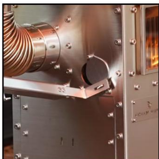
Shut the ignition port
