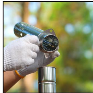
Install spark arrester and fixed ring
