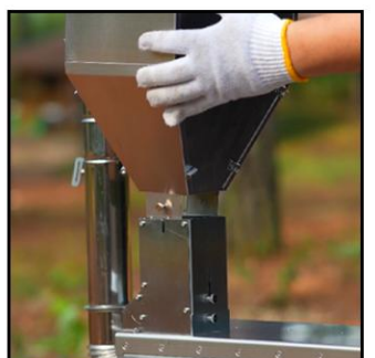
Insert pellet hopper into pellet tube
