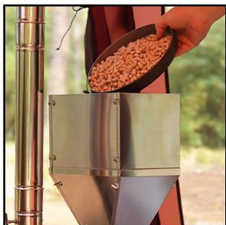
Add pellet into the hopper
