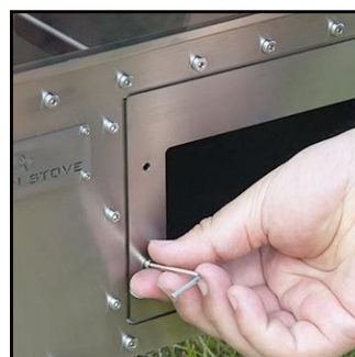
Take out the two screws on left side of oven
