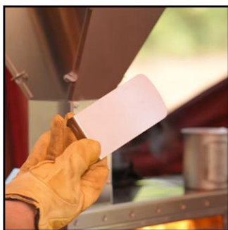
Insert the blocking pin to the gap between the fuel tank and pellet tube
