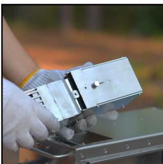
Insert pellet cage into pellet tube
