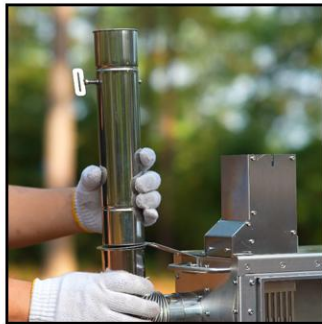
Install regulating chimney tube
