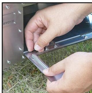
Install back the retainer plate
