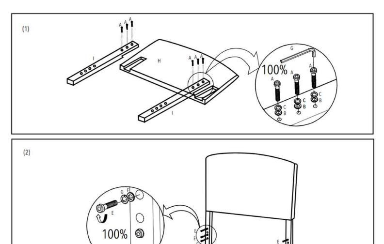
Ensure that all bolts are tightened before use. Check and tighten all bolts periodically throughout use of the product.
