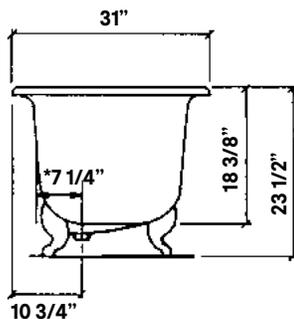
\*8 1/2" C.C. waste/overflow to drain
