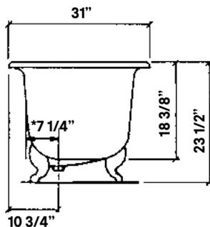
\*7 1/4" C.C. waste/overflow to drain
