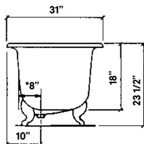
\*8" C.C. waste/overflow to drain
