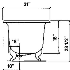
\*8" C.C. waste/overflow to drain
