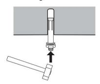
If installing into concrete/brick, tap in the expansion bolts. Expand them enough to hold in place by tightening the nuts, do not fully tighten yet!
