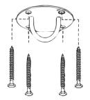
If installing into wood, position the round eye pad over the pilot holes and drive the screws into the pilot holes.
