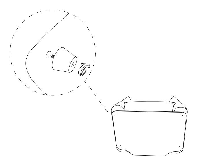
> Position the product bottom-side up and simply screw the legs into the pre-drilled holes as illustrated
