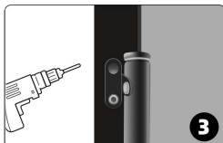
Knock out the rivets with an electric drill
