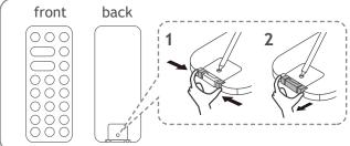
To remove the battery holder, hold the top dot with a ballpoint pen or a round-shaped tool. Then, push on two sides and pull the battery holder out simultaneously.
