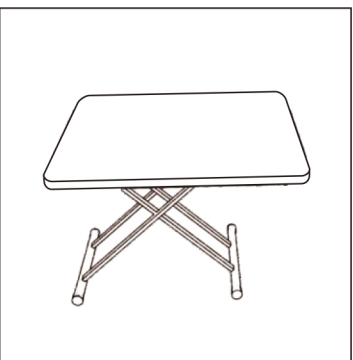
STEP4: Rotate and open the table top to increase the size of the table top 100X110cm
