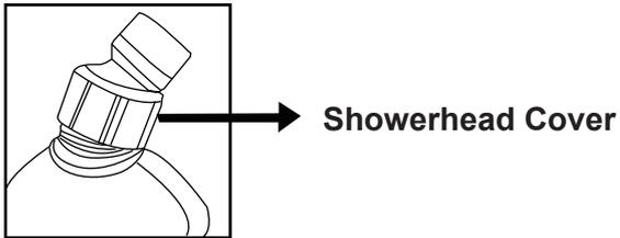
Remove the Showerhead Cover by turning it counter-clockwise.
