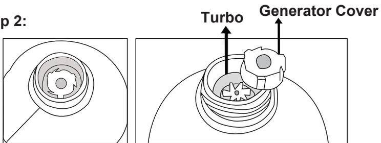
Remove the Generator Cover. Clean the Turbo and turn the Turbo a couple turns.
