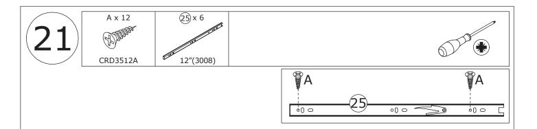
Fix track 25 to plate 17, 18, 19 and 20 with screw(A) as shown.
