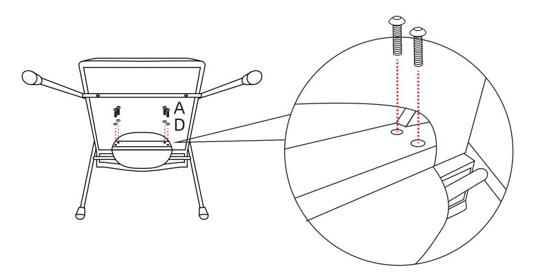
4. Open the zipper at the bottom of the seat cushion, use B screws to fit D washers, and install the seat cushion on the backrest
