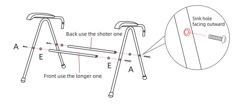
1. Install the iron frame together with screws A as shown in the diagram.
