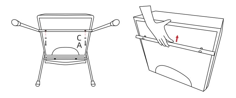
5. Pull up the zipper, then use the A screw to cover the C gasket, and install the seat cushion onto the iron frame
