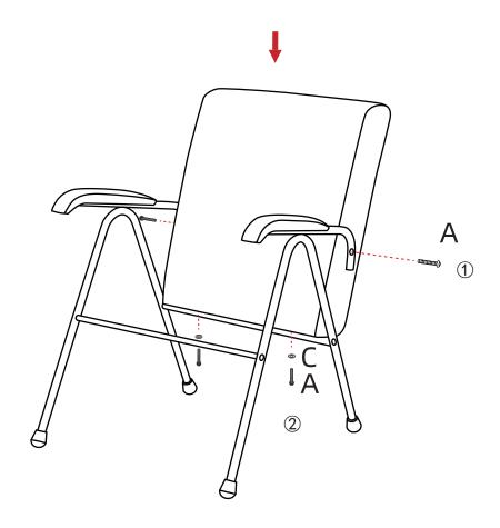
2、Place the backrest on the back of the iron frame, first use screw A to install the armrest position ①, then use screw A to install the seat cushion position ② with washer C
