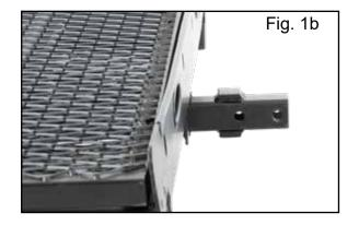
**Step 3.** Tighten jam nuts with 17mm or 11/16" wrench until holes line up from carrier and hitch height adapter.
