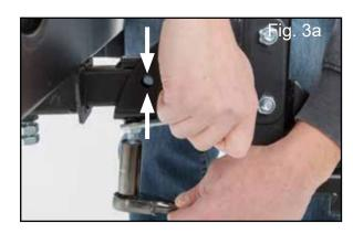
**Step 5.** Remove pin with clip to fold carrier vertically. Replace pin in top hole to secure carrier in vertical position.
