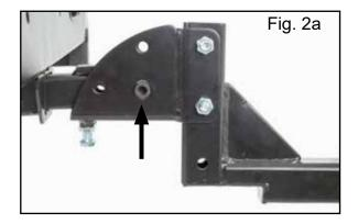
**Step 4.** Insert pin with clip from scooter carrier to secure in position.
