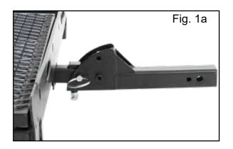
**Step 2.** Install scooter carrier to hitch height adapter with hex head pivot bolt and lock nut from carrier. Tighten bolt.
