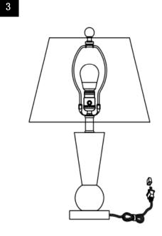
Step2 Insert the bulb(G) into the socket(C).
