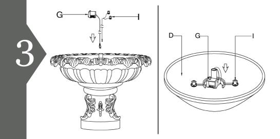
Place lower column (B) into reservoir (D) and twist it clockwise to secure.
