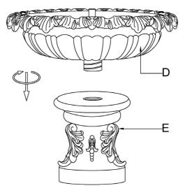
Feed pump cord and light cord through plastic tube, make sure the cords exit out from notch on bottom of base (E).
