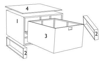
2. Attached Leg frames (2) to Frame (1) by using M6x25mm bolt (A) with Washer (B), and fasten with Allen Key (C).
