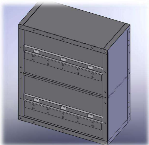
Back Panel View of Wall Cabinet shows 6 flat hooks that allow the Cabinet to hang on two Wallhanging Brackets.
