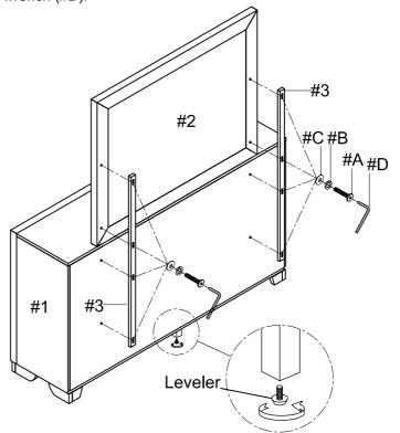
Adjust the leveler according to the ground level. To lower or to raise the slat support leg, you need to turn the leveler clockwise or counterclockwise, respectively.
