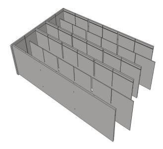
Step 1: Attach Top, Bottom, and (2) 5/8" thick shelves into a Side piece using (8) supplied Hex screws and Allen wrench provided. Back grooves in Top and Bottom, -cuts that go all the way through from short end to short end, align with 3/8" deep back groove in Side piece. Back grooves face inwards torwards middle of Side piece. Slots in 5/8" thick shelves also point torwards 3/8" deep back groove in Side piece.
