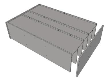
**Step 5:** Attach second **Side** piece using **(8)** supplied Hex screws and Allen wrench. Overhang on backs past Top, Bottom, and shelves will fit into deeper 3/8" back groove of second Side piece.
