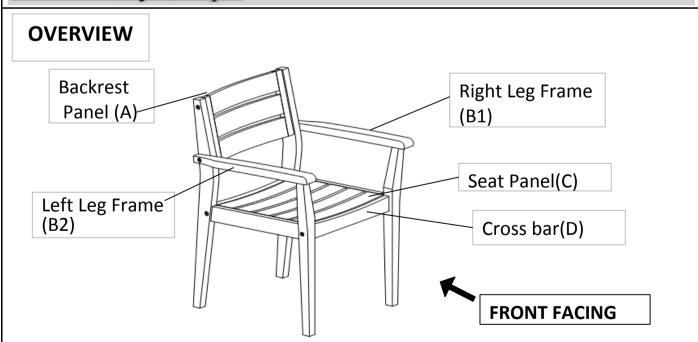
This Chair has multiple parts and may require up to some 30 minutes to assemble. To give you an overview of the Chair, the above picture to assemble to help you put the various parts into perspective. Please read through the instructions here below to familiarise the parts and steps before assembly.
