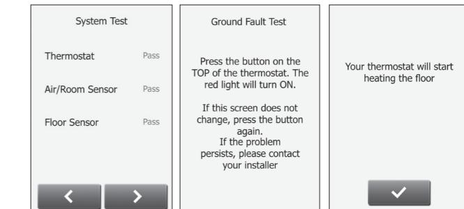
Perform system and GFCI/EGFPD tests. Once thermostat setup is complete, confirm "Your thermostat will start heating the floor" to complete the startup wizard.
