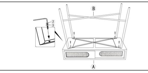
Attach Legs(B) to Table Top(A) using Bolts(2) and Flat Washers(3) with the Allen Key(4)
