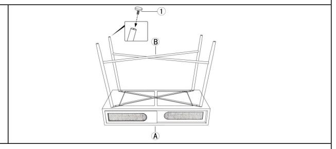
Attach the Adjustable Levellers(1) to the Legs(B) by hand.
