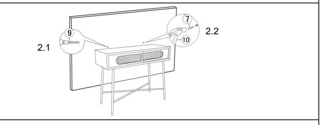
2.1)Drill two holes on the wall at the same height as the Restraint Straps(®) on the Table using a Power Drill(9).
