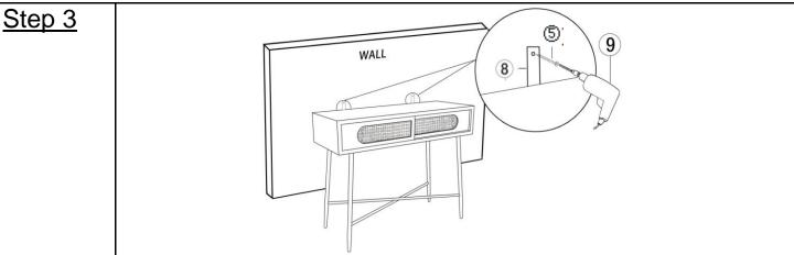
Attach the Restraint Strap(®) to the Wall Anchor (⑦) using a Screw(⑤) and the Power Drill(⑨) Your Table is ready for use.
