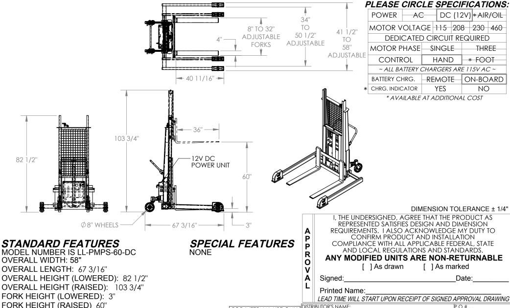
FORK CAPACITY: 1200 LBS (EVENLY DISTRIBUTED) FORKS ARE 1 1/2" THICK X 4" WIDE X 36" LONG MAXIMUM FORK SPREAD: 32" 12V DC POWER UNIT CONTROL PENDANT W/ 8' CORD NOT SHOWN ALL STEEL CONSTRUCTION (ASTM A-36 MIN) FOR INTERNAL USE ONLY
