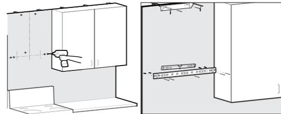
**Caution:** One of the wood screws(#10×2 9/16"(ST5×65mm)) for duct bracket must be fastened to the wooden beam.
