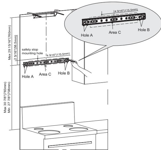
**Caution:** one of the wood screws(#10×2 9/16"(ST5×65mm)) for main engine must be fastened to the beam.Screws must be fixed at hole A and B in the drawing; also wood screws(#10×2 9/16"(ST5×65mm)) must be fixed at bracket bores with corresponding wooden stakes in area C.
