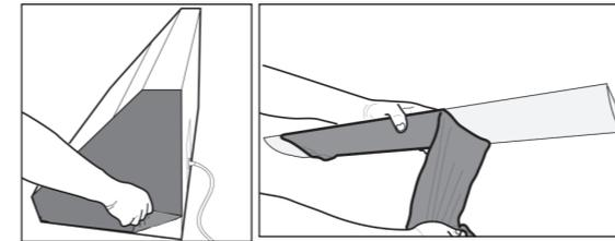
7. Lift and position the hood onto the mounting screws. Make sure the hood is stable and leveled by using a spirit level. Install the safety buffer baffle above the hood(The safety block is provided in the accessory bag in the packing box of the decorative cover assembly.).
