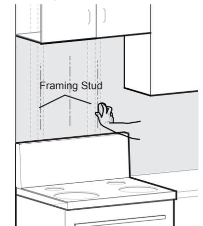
3. Locate the duct bracket. Determine the central point and mark the centerline on the wall where the hood will be installed. Also, mark the point where the central line and the top cabinet meet. This is the location, in which to secure the bracket. Mark screw hole locations on the wall. The upper edge (the fixed surface
