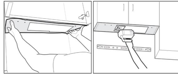
**Caution:** Wear safety goggles when drilling. In case of batten at the wall facing the bottom plate, the rear wall side of the paper template shall be cut as per the thickness of the batten. If it is necessary to fix the hook on the tile, the "Rear Wall" side of the hole-drilling template should be attached to the bottom of the upper cabinet, using the tile surface as a reference.
