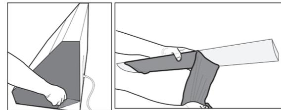
7. Place the seal (notch downward) at the air outlet of the machine and fix the outlet housing with 4 outlet-housing bolts of #8×3/4"(M4×18mm).
