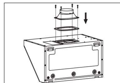
8. Lift and position the hood onto the brackets at the top of the backside while keeping an angle between the wall and the hood, and then push the hood against the wall tightly. Secure the duct to the duct cover and seal the connection
