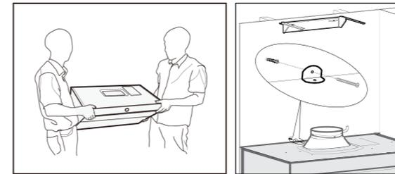
**Caution:** Two installers are required to ensure safe installation. Please install the safety stop as required. The main function of the safety stop is to prevent the range hood from being lifted up accidentally, which will cause it to unhook and potentially fall.
