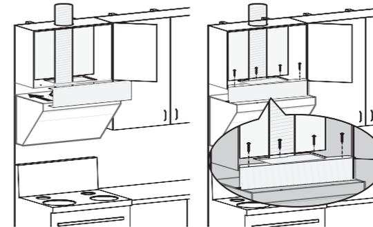
10. Make sure the hood is leveled. Install the Grease Cup, and plug the appliance for a test run.
