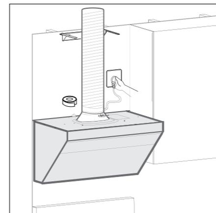
**Caution:** Please run the machine and test if the smoke pipe leaks air after it is sealed with aluminum foil tape. The smoke pipe should be able to be straightened as much as possible.
