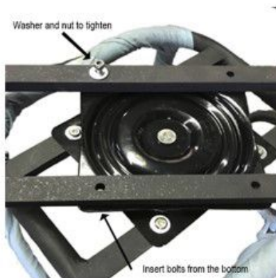
5. Insert bolts from the bottom of the top swivel plate and insert washer and nut from the top to tighten.
