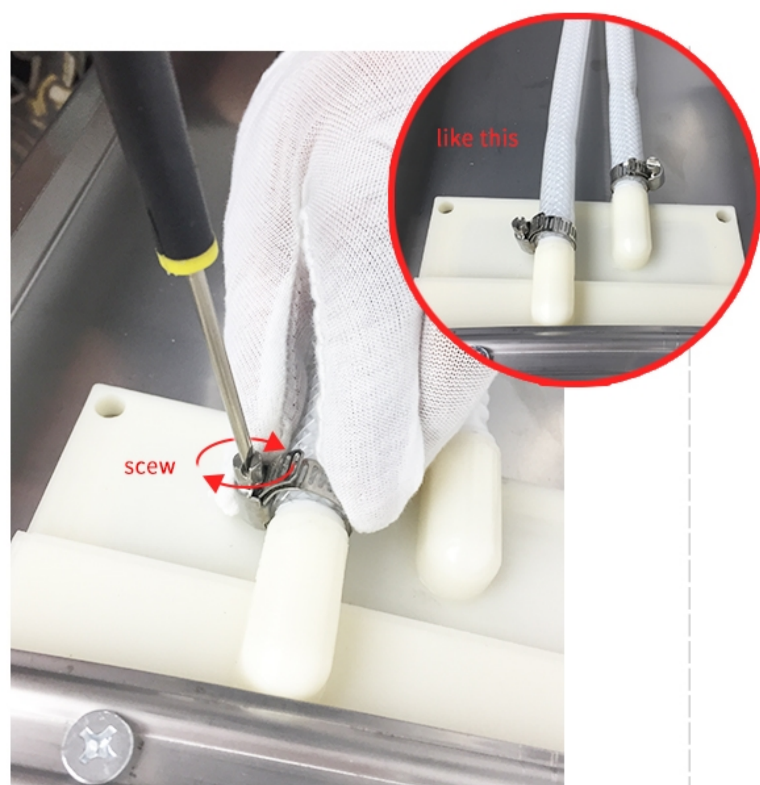
(13) screw the screw and fix the hose
