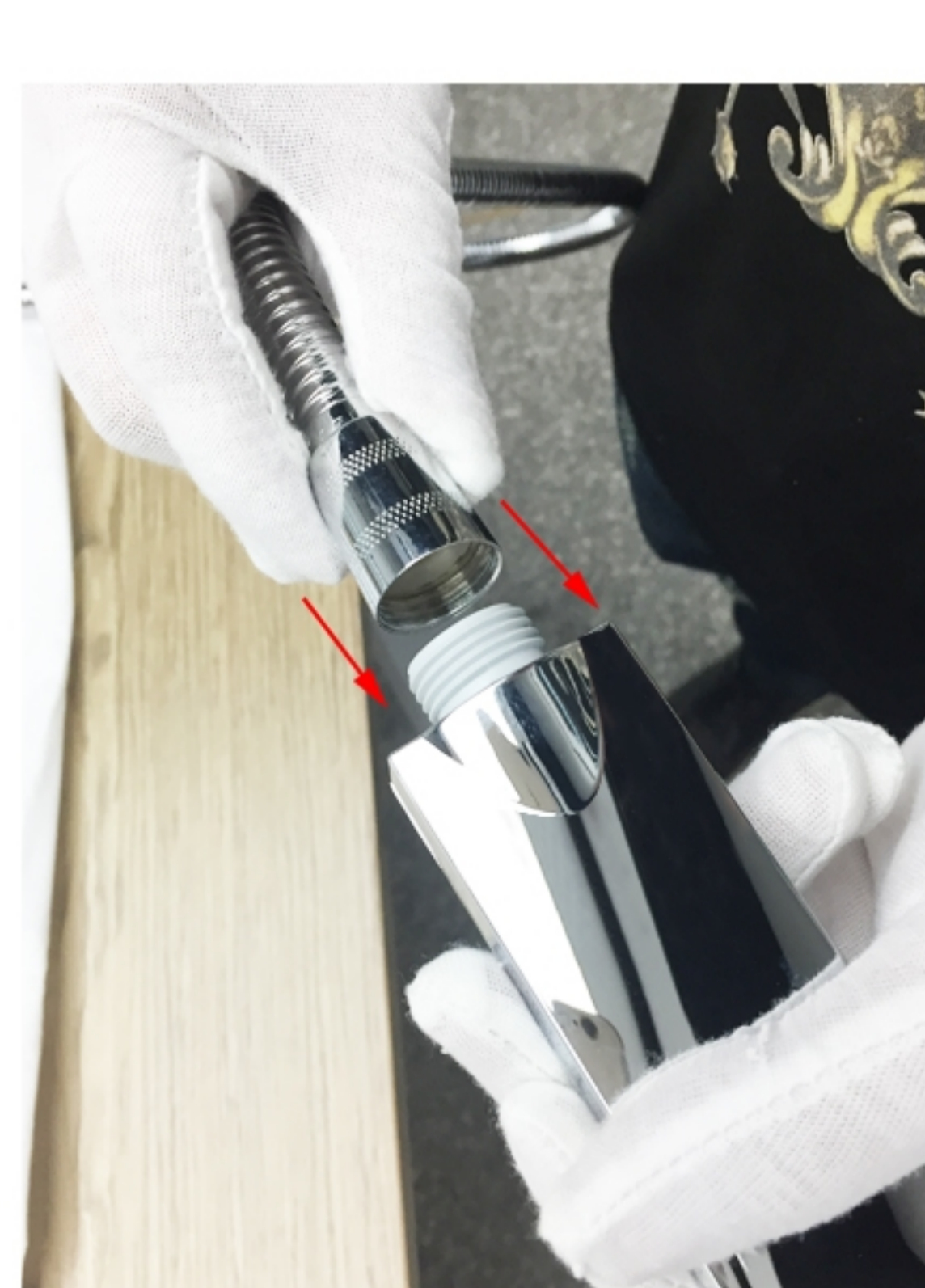
(14). screw the other side of hose on the hand spray
