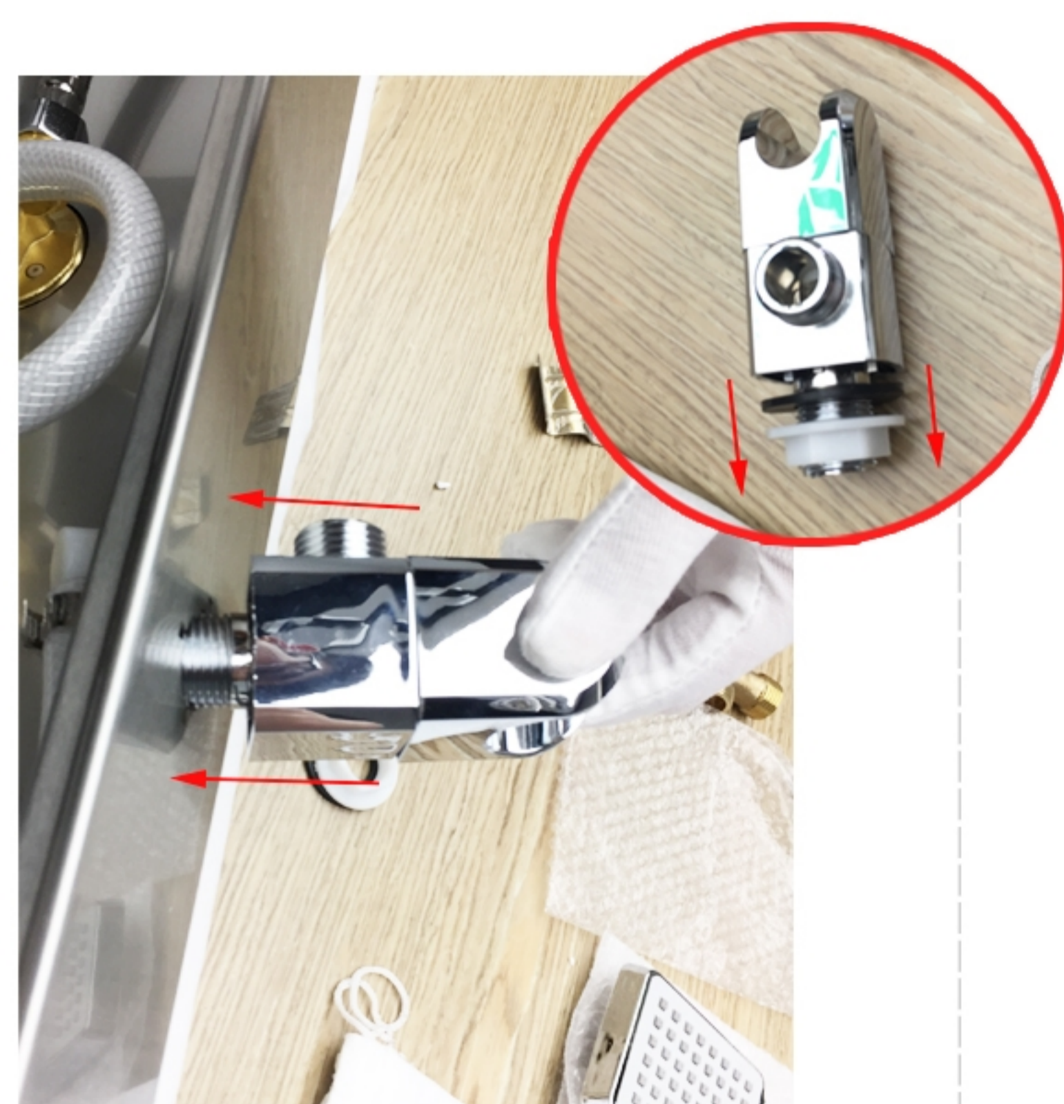
(6). take away the white screw nut and black gasket, then install the left part.
