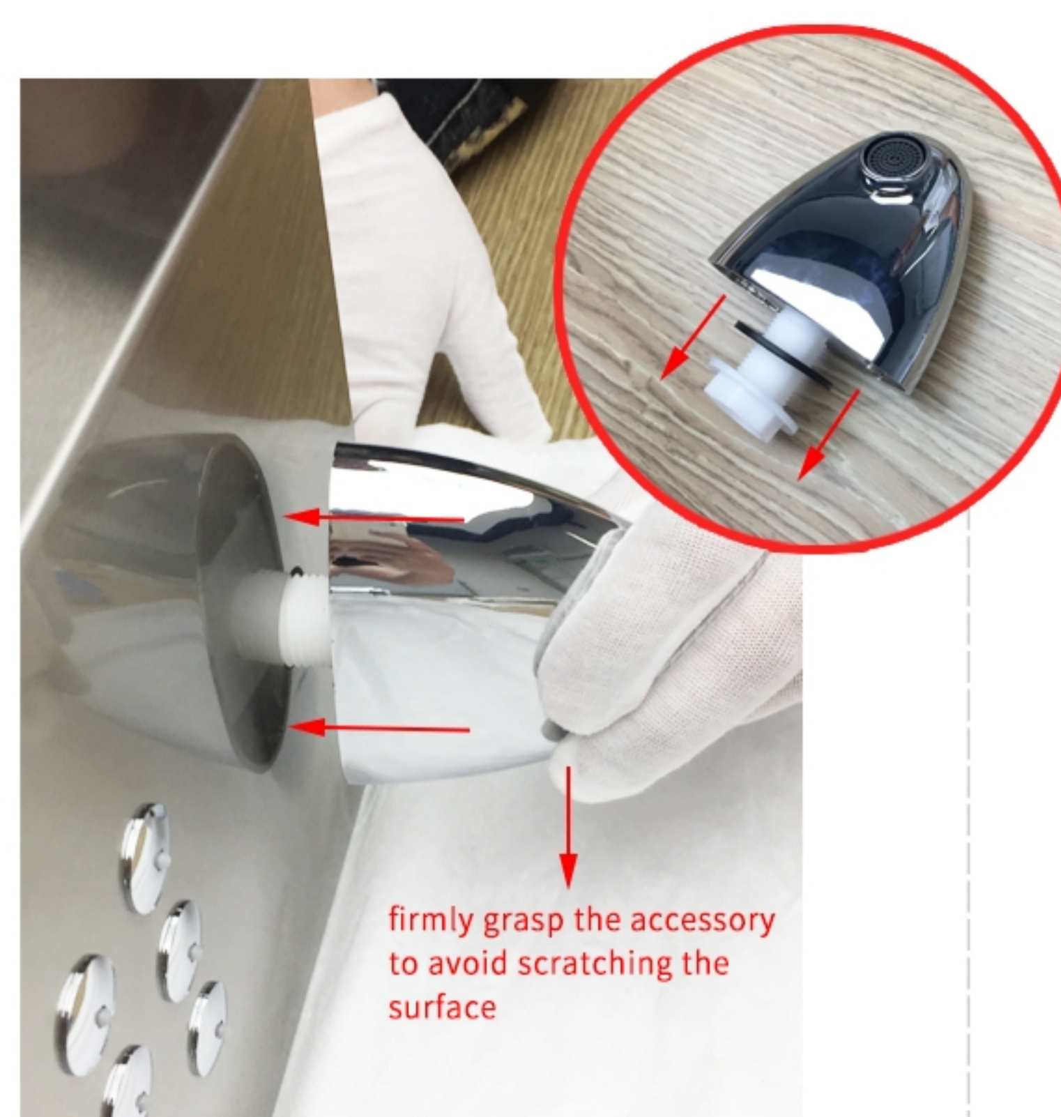
(3). take out the white screw nut and black gasket, then install the water nozzle.
