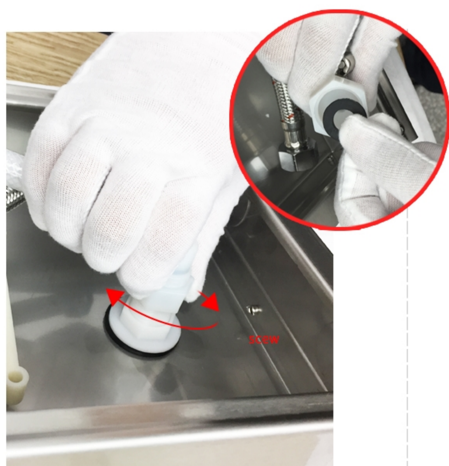
(5). put the gasket into the screw nut and screw them on the water nozzle.
