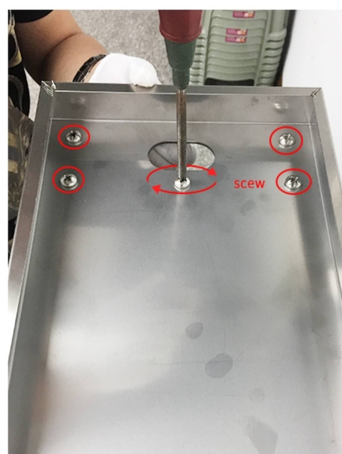
(10). screw the five screws
