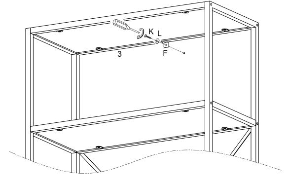
(Optional) Secure unit to the wall using screws (K) and washers (L) at the installation points of wall plugs (J) from previous step.
