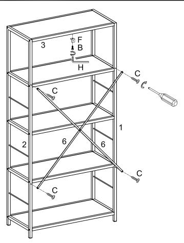
Secure cross beam assembly to frame using screws (C). Secure angle iron (F) using bolt (B).
