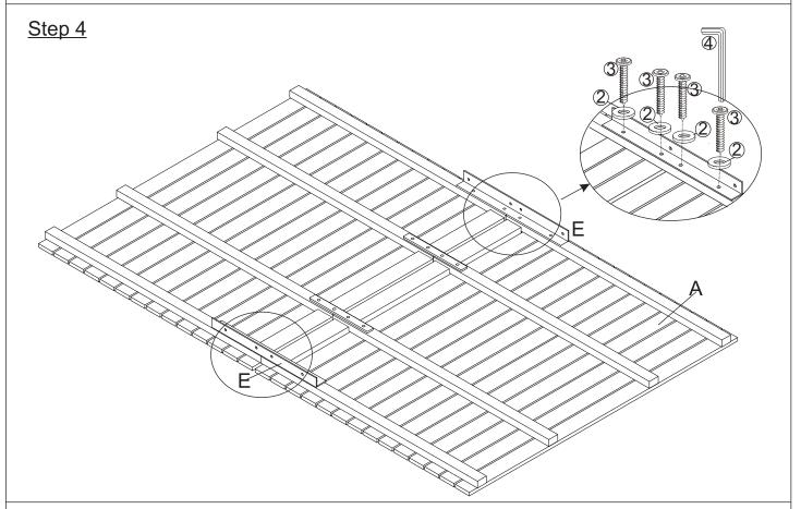
Place Side Support Bar (E) to the housings of Table Top (A), secure by using the Screws (3), Washers (2) and Allen Key (4), as shown in the picture. **Do not fully tighten the Screws.**
