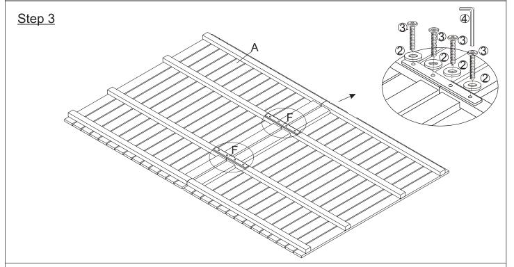
Place Middle Support Bar (F) to the housings of Table Top (A), secure by using the Screw (③), Washers(②) and Allen key (④), as shown in the picture. **Do not fully tighten the Screws.**
