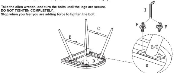
Align Center Cross Bar(E) to Left Leg (B) and Right Leg (C) then tighten with Bolt with Lock Washer and Flat Washer (F) and Allen Wrench (J).
