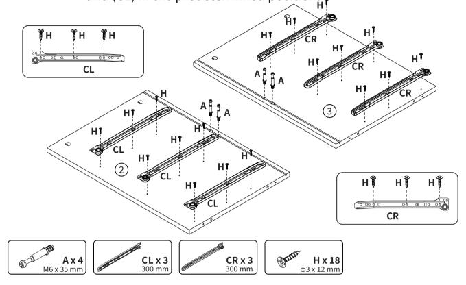
**Step 2** As shown below, use screw (H) to lock rail guide (CR) and (CL) on two side of part 4 in the predetermined position.
