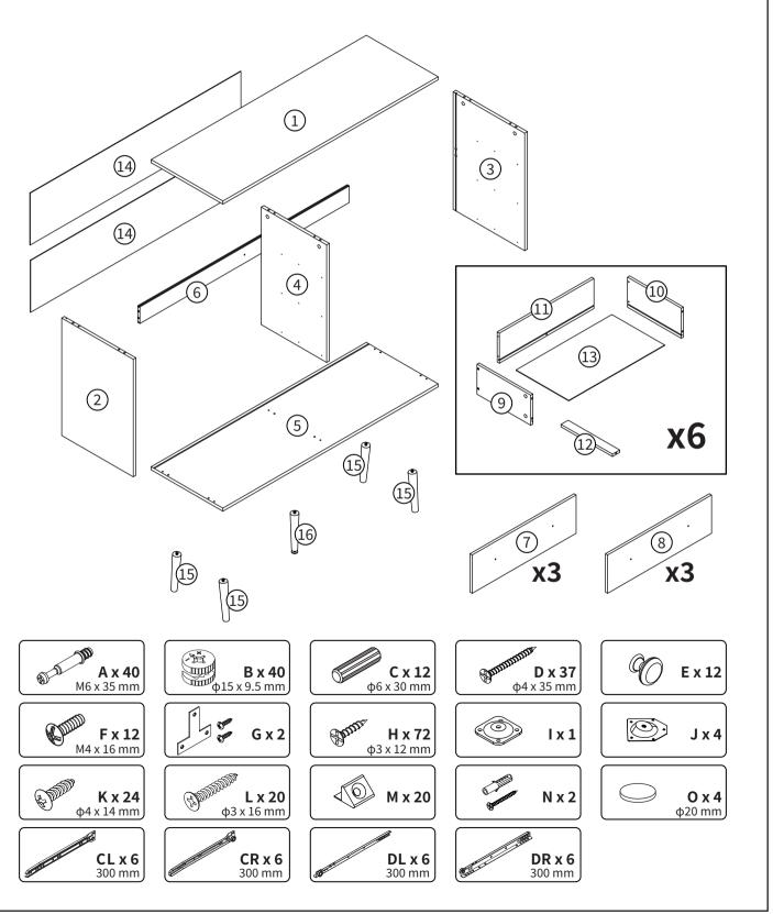
As shown in the figure below, use screw (A) to install on board parts 2 and 3, and then use screw (H) to lock rail guide (CR) and (CL) in the predetermined position.
