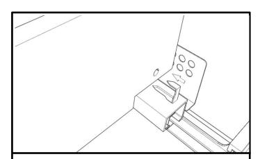
Ensure that the hook on each runner profile fits into the corresponding holes on the drawer back panel.
