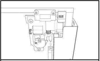
Insert the drawer on the extended runner. To secure the drawer clips with the runner, push the drawer in. Upon successful locking, a click can be heard.
