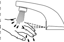
3. When hands are moved away from the OPTIMA® Sensor, the loss of reflected light initiates an electrical signal that deactivates the Solenoid Valve, shutting off the water flow. The Circuit then automatically resets and is ready for the next user.
