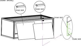
6. Install the glass lock: Attach glass lock part A to the inner slot of the glass and tighten the screw, then lock the other part, B.
