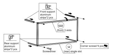
2. Install the back panel, left and right side panels, and front panel (Note: The front panel should be installed in the last slot).
